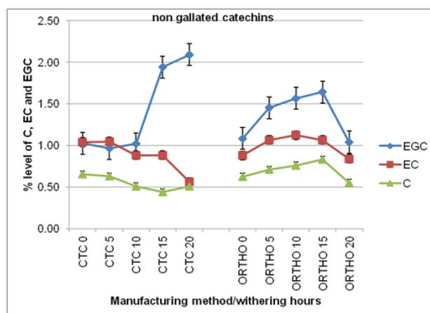
Figure 2. Effect of manufacturing method and withering duration on non gallated catechins percent levels. Each value is a mean of three replicates. Bar means  $\pm$  standard error. Key CTC, Cut Tear Curl; ORTHO, Orthodox; C, Catechin; EC, Epicatechin; EGC, Epigallo catechin.
